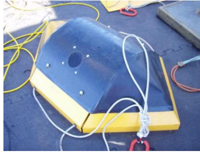
Figure 1A. High flow mooring. The circle near the top of the cover is an acoustically transparent window (Source: JASCO Applied Sciences)
